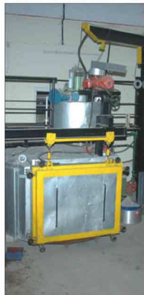
EPOXY Casting Plant
