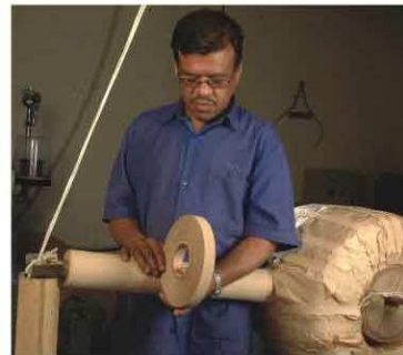
Taping of PT Coil
