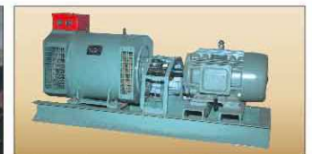
Induced Generator Set for Voltage Transformer Testing
